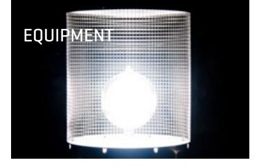
Based on a proprietary light engine, our solar simulators deliver perfect and continuous artificial sunlight 24/7, allowing for accurate stability and performance assessments of solar cells at laboratory and industrial scales.
